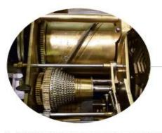
The writing hand is powered by two clockwork motors.
