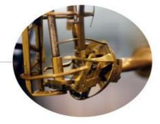
The styluses in turn drive a series of rods, providing motion. There is a separate stylus for each direction: forward and back, side to side and up and down.
