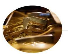
Each of the writing hand's 72 cams has a pattern cut into its edge corresponding to specific arm movements.
